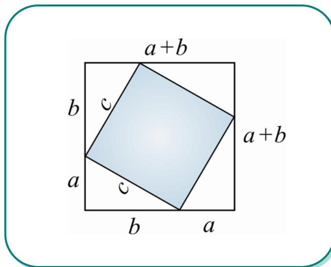
$$\begin{aligned} \text{Área Total: } & c^2 + 4 \cdot \left( \frac{a \cdot b}{2} \right) = (a + b)^2 \\ \Rightarrow & a^2 + b^2 = c^2 \end{aligned}$$
